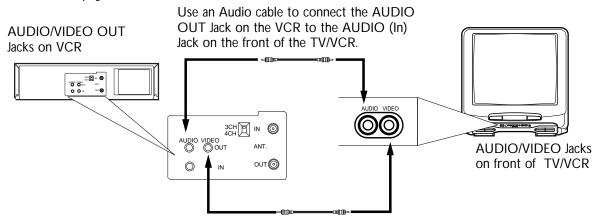
Use a Video cable to connect the VIDEO OUT Jack on the VCR to the VIDEO (In) Jack on the front of the
